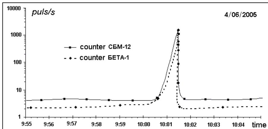
**Fig. 4.** An example of a burst of the count rate of a  $\beta$  source mounted at the focal point of a mirror with parabolic surface. Radiation from a  $^{60}\text{Co}$  sample was registered by means of two independent Geiger counters [3, 17].
