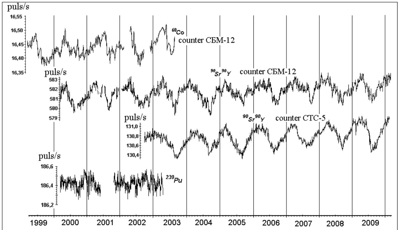
**Fig. 3.** Count rates for  $^{60}\text{Co}$  and  $^{90}\text{Sr}$ - $^{90}\text{Y}$  sources as measured by G-M counters, adjusted for decrease in the radioactivity with half-lives of 5.26 and 27.7 years, as well as count rate for a  $^{239}\text{Pu}$  source, as measured by a silicon detector [3, 16]. Curves corresponding to  $\beta$  sources exhibit an easy to see annual rhythm, whereas measurements of alpha decays reveal no periodic variations.
